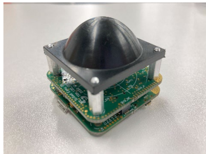
Radar devices used as Sub-THz generator
